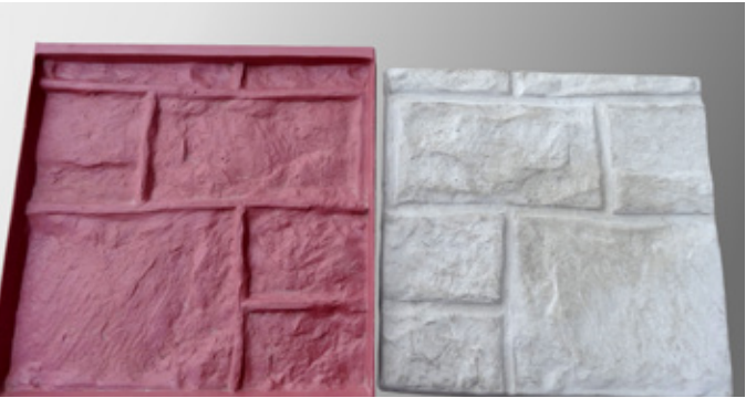
Carity made of GM 965-55, concrete casting
