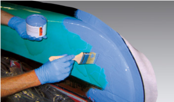
Application of gel coat OH 6-1
